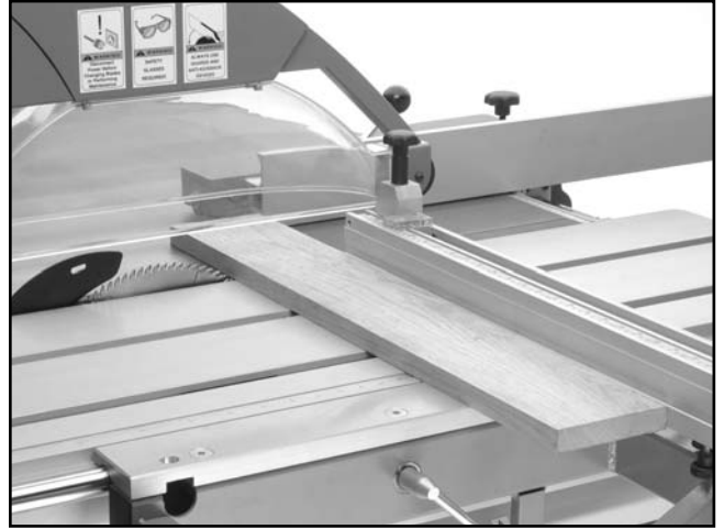
Figure 71. Crosscutting workpieces using the rip fence as a cut-off gauge.
